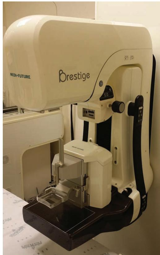
Fig. 1. Add-on stereotactic device attached to a mammography unit.
