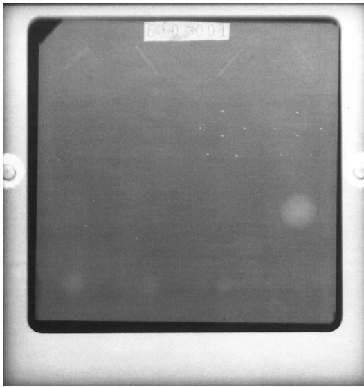
Fig. 2. Passed phantom image that the total score is 11 (fiber-4, groups of specks-3, masses-4) and optical density is 1.43.
