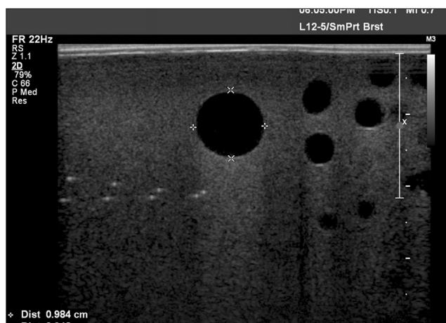
Fig. 6. Evaluation of anechoic object imaging. A 1 cm sized anechoic mass and 3 mm and 5 mm sized anechoic spheres can be used for anechoic object imaging test in this phantom. The image demonstrates anechoic mass with a round shape and circumscribed margin. The difference between width and height is 3.6 mm, less than 15%.
